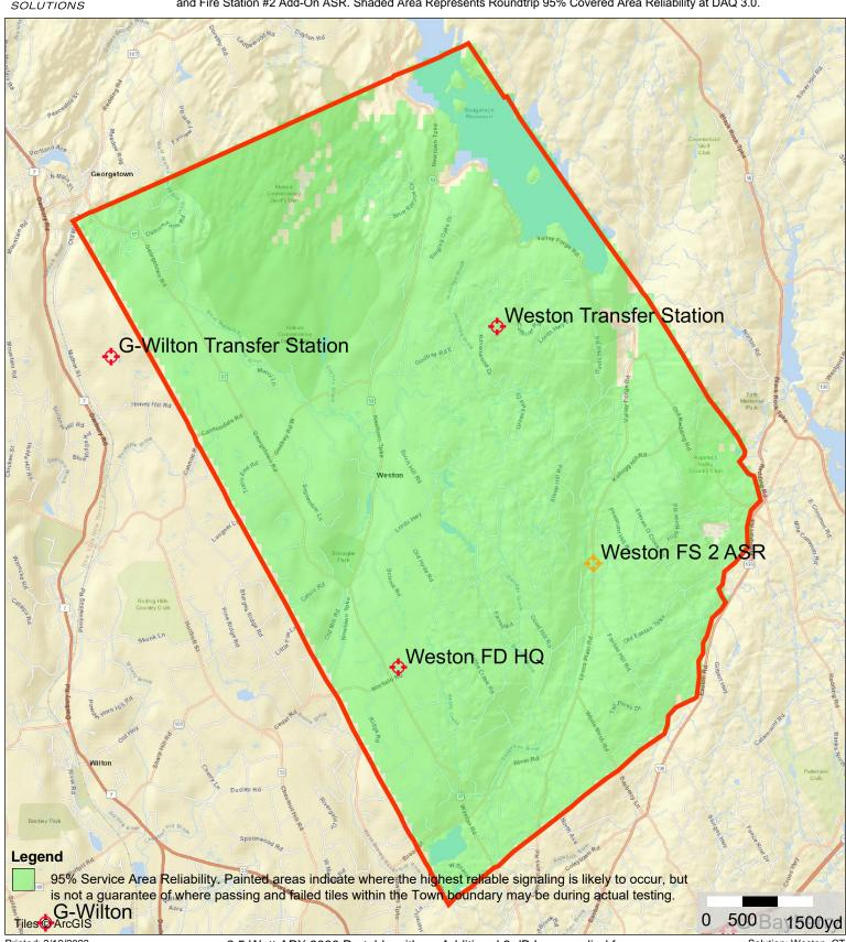
Printed: 3/10/2023 System version: 3.0.3.0 2.5 Watt APX 8000 Portable with an Additional 8 dB Loss applied for Building Penetration with the Standard XE All-Band Antenna in a Swivel Case on the Hip with a Remote Speaker Microphone for Transmit and Receive.
