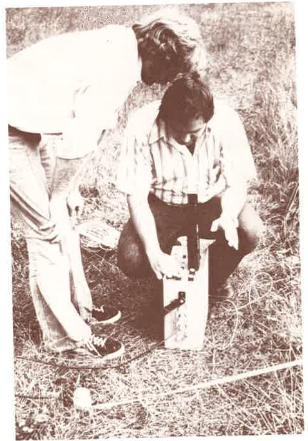
Depth to bedrock can be determined in the field with the aid of seismic testing. The geophone on the ground in the foreground measures the amount of time a shock wave requires to travel through the ground at various depths. The wave velocity indicates the material through which it has traveled.
