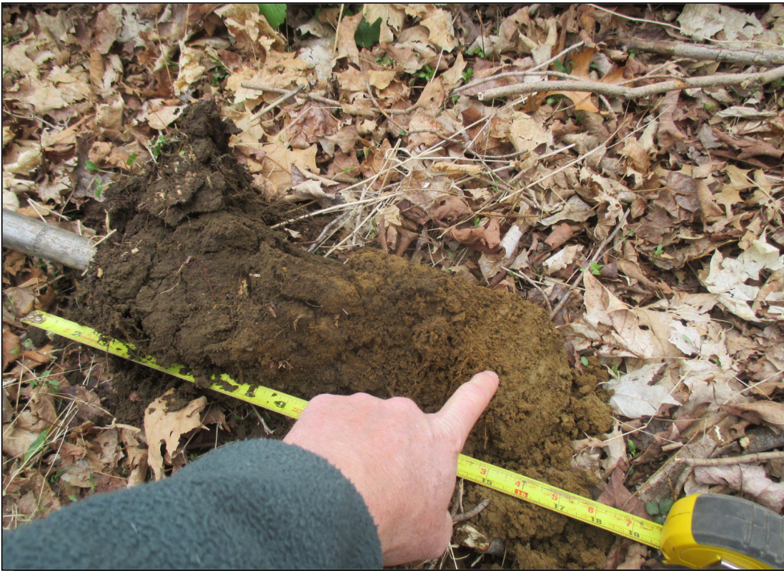
Photo 3: View of soil profile in vicinity of underground detention system (Note redoximorphic features at 16-inches) (JMM photo taken 4/18/2022)
