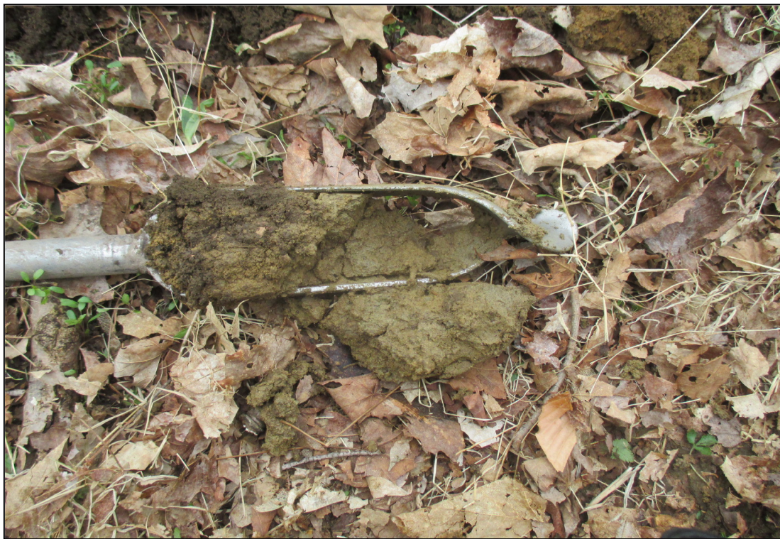
Photo 4: View of redoximorphic features at 23-inches (JMM photo taken 4/18/2022)
