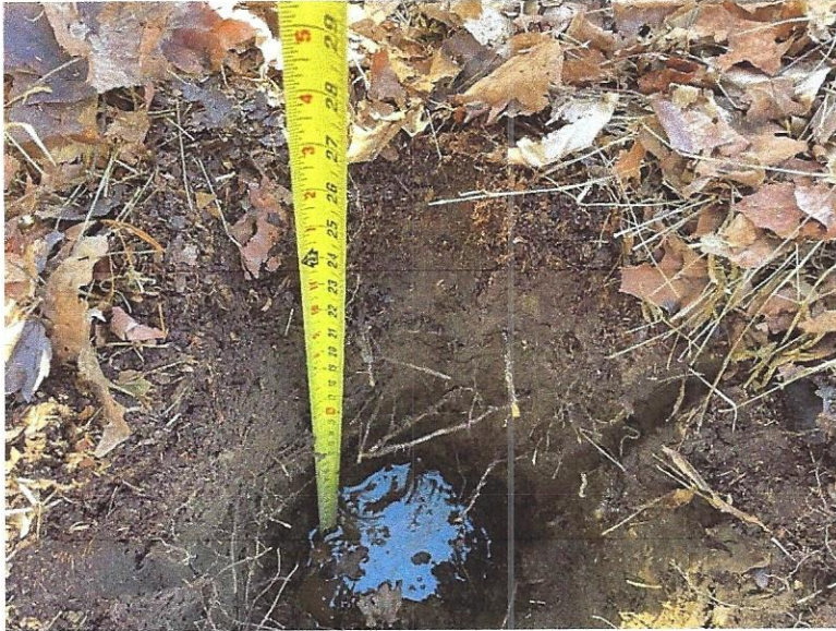
Figure 1 - Groundwater at 23" in hand hole
