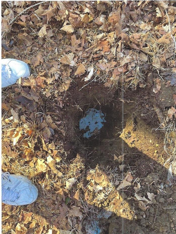
Figure 2 - Groundwater in hand hole
